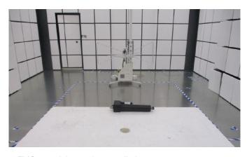
EMC test air immunity or radiation test
