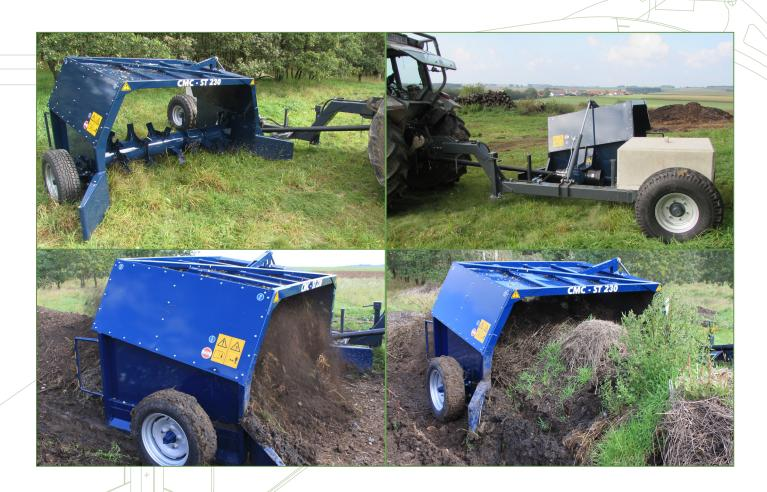
The new **CMC ST 230** offers high performance with compact design. The machine creates perfect mixing and ventilation results for tractors of minimum 30 hp. With a net tunnel opening of 2.3 m the machine can turn compost windrows up to a width of 2.6 m. Built on a trailer, in the proven system, the machine
