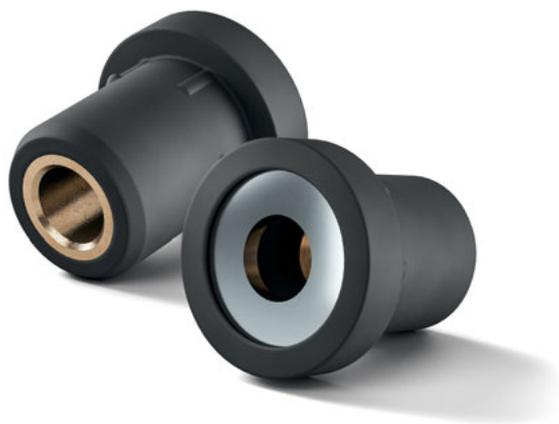
The SITEC® Rivet without internal thread offers further joining options. Since a fastening thread (such as a weld nut) is required on the other component, larger wall thicknesses (or spacings) can be spanned and the components can be joined with a damping effect.
