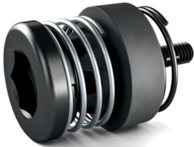
The purpose of the SITEC® Spring fastening element is to isolate vibration. Individually adjusted spring rates eliminate the vibration of large applications, for example in a vehicle. The assembly is delivered in two parts and is pre-assembled on your application without the use of tools so that it cannot be lost during transport. When it is then screwed together, the fastener can compensate radial tolerances of up to  $\pm 1$  mm.
