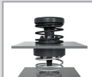
Screwing of the mounting part to the thread of the receiving part with the screw element
