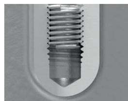
Blind hole for HELICOIL® with tang according to DIN 76 Part 1 (normal case)
