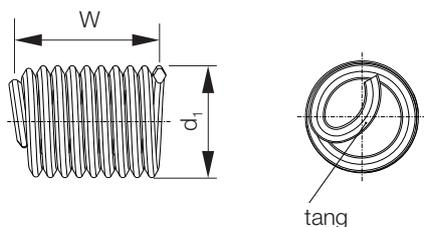
The control values of not installed thread insert free running are W and d<sub>1</sub>.
