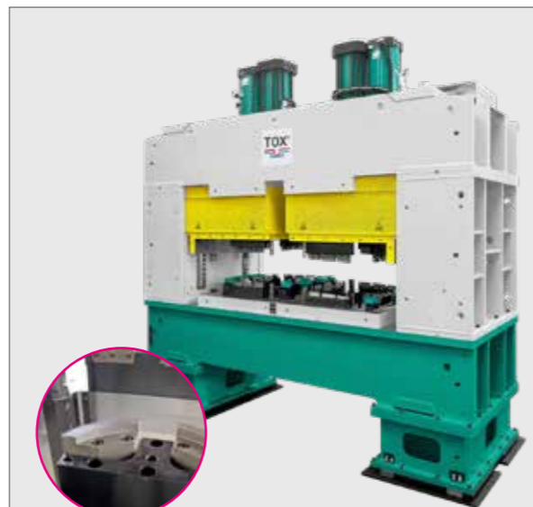
TOX® Press with punching tools It punches sunroofs-cutouts into sheet metal.
