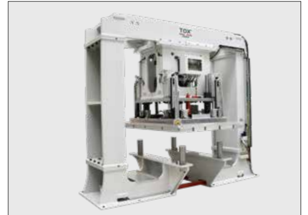
TOX® Press system series MAG for production of battery packs.
