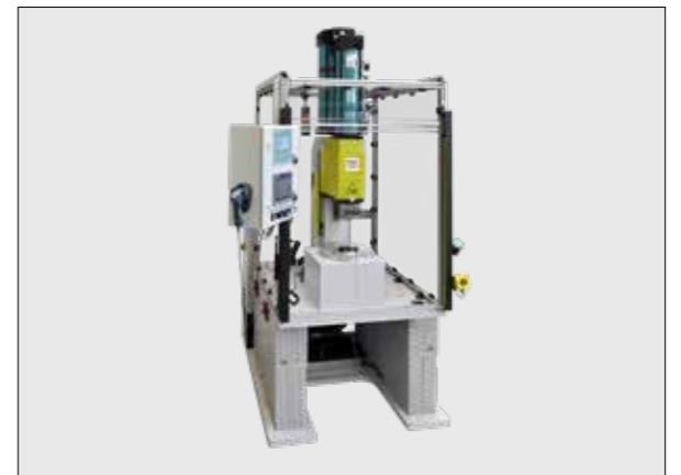
TOX® Press with a multi point clinching tool.
