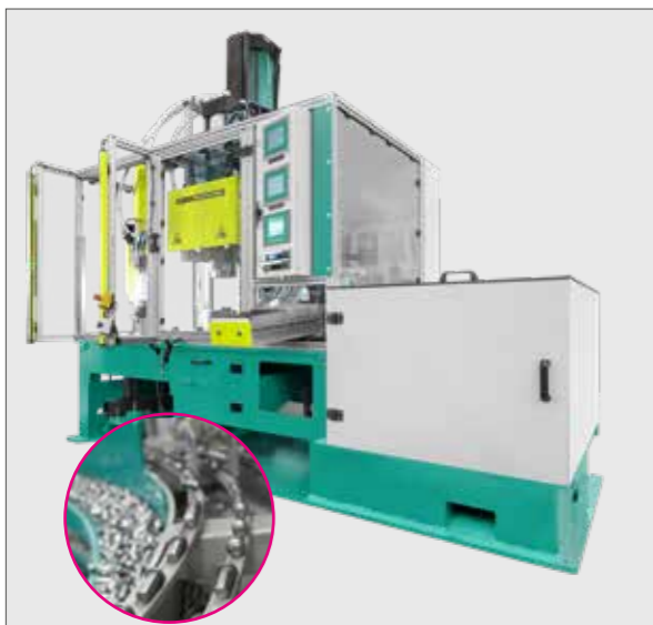
TOX® Press that presses in 16 rivets in one step.
