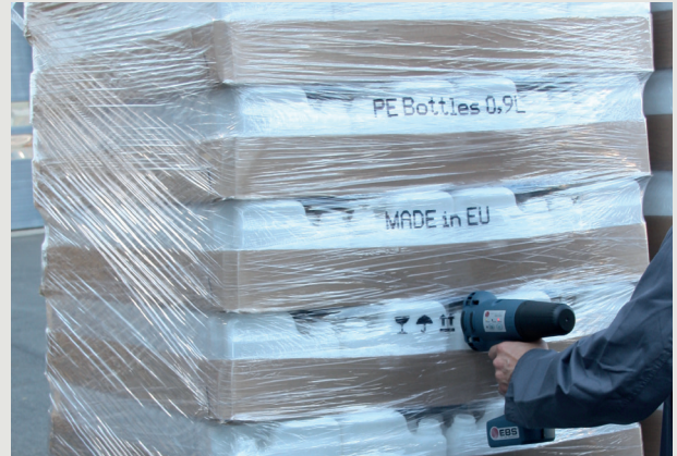
→ Stretch Film printed with black universal ink (ethanol); large spacing wheels.
