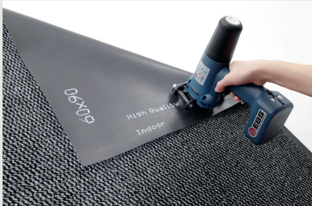
→ Rubber printed with white pigmented ink (ethanol); 4-wheel stabilizer.
