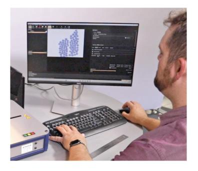
The included **perClass Mira Software** enables even non-domain experts to rapidly build solutions for automatic segmentation of hyperspectral images. The perClass Mira Software controls all acquisition hardware, provides an intuitive analysis interface, and enables model deployment with visual feedback—no switching between acquisition, analysis, and deployment interfaces.
