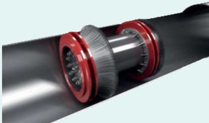
Figure 12: Example of Pipe Cleaning Pig <sup>54</sup>
