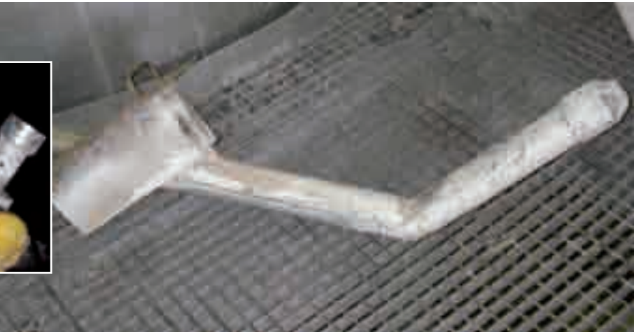
Twin-fluid nozzle lances in an existing system, with tables for the frequently necessary disassembly and cleaning of the nozzle lances
