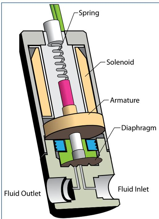
The valves use a flexible diaphragm to isolate the solenoid actuation mechanism from the fluid path. Isolation Valves are available in three different configurations; normally closed, normally open and 3-way. When the valve is energized, the solenoid retracts the armature that is attached to a flexible diaphragm. In a
