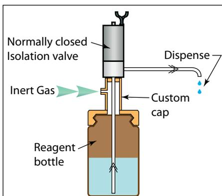
Maintaining a repeatable dispense of aggressive (and often very expensive) reagents into an analytical instrument can be problematic with conventional pumping equipment.
