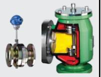
Type IPD system - explosion suppression and isolation systems detect the earliest stage of a deflagration by sensing the pressure wave that comes ahead of the flameball and uses the signal to activate delivery of an extinguishing agent
