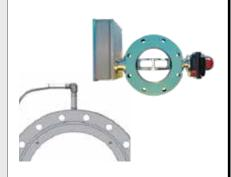
Convenient, Economic, Corrosion Resistant Graphite disks are made from impregnated graphite offering low burst pressure and excellent corrosion resistance. BS&B graphite disks are supplied with integral gaskets for direct installation between international pipe flanges. The replaceable element range is installed in graphite or stainless steel safety heads before installation between pipe flanges.
