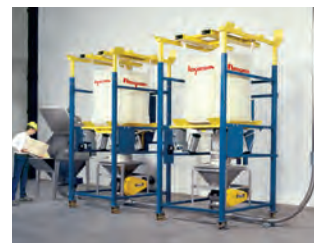
The Loss-of-Weight Batching System at left discharges one or more bulk bags while weighing the material and conveying the batch directly to any process vessel. Load cells transmit the amount of weight lost to a controller, which stops the conveyor once the target batch weight has been reached. The system at right conveys material from two Flexicon bulk bag dischargers into a filter receiver which discharges into a blender. The manual bag dump station allows the addition of pre-weighed minor ingredients to the batch.
