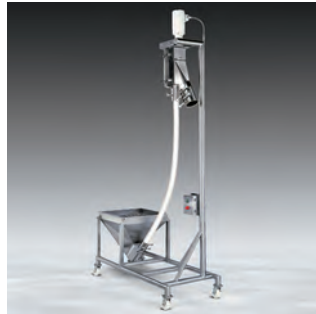
Sanitary Flexible Screw Conveyors are totally enclosed, preventing plant and product contamination. The inner screw connects to the drive motor beyond the material outlet, eliminating material contact with bearings. Tool-free disassembly.
