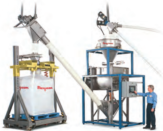
Flexicon's Self-Contained, Gain-in-Weight Batching and Blending System conveys bulk ingredients from multiple upstream sources, weigh-batches, blends and discharges the material into a surge hopper, and transports it to a TWIN-CENTREPOST™ Bulk Bag Filler. The system is offered with Flexicon Flexible Screw Conveyors (shown), FLEXI-DISC™ tubular cable conveyors or PNEUMATI-CON® Pneumatic Conveying Systems.
