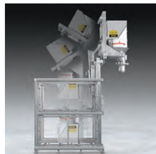
Sanitary TIP-TITE® Drum Tipplers allow loading, sealing, tipping and discharging of drums with no dusting by forming a dust-tight seal between a drum discharge cone and a gasketed receiving ring fitted to existing process equipment or the lid of a hopper.
