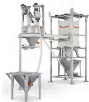
The Gain-in-Weight Batching System at left weighs a major ingredient supplied in bulk bags, and a minor ingredient dumped manually. The controller starts and stops the conveyors to weigh each material in sequence, and actuates a slide gate valve to discharge the batch. The system at right conveys material from four BULK-OUT® bulk bag dischargers to a weigh hopper which discharges into a blender. Blended batches can be discharged into shipping containers (shown) or process equipment.
