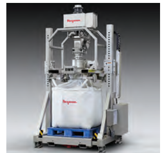
Sanitary TWIN-CENTREPOST™ Bulk Bag Fillers provide a dust-tight, inflatable bag spout seal, a feed chute air-displacement port for dust-free filling, and four-sided access for easy connection of bag straps and bag spout, and rapid wash down.
