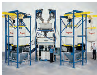
The Gain-in-Weight Batching System at left weighs a major ingredient supplied in bulk bags, and a minor ingredient dumped manually. The controller starts and stops the conveyors to weigh each material in sequence, and actuates a slide gate valve to discharge the batch. The system at right conveys material from four BULK-OUT® bulk bag dischargers to a weigh hopper which discharges into a blender. Blended batches can be discharged into shipping containers (shown) or process equipment.
