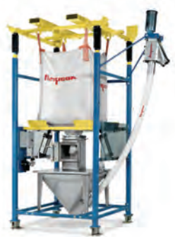
The Loss-of-Weight Batching System at left discharges one or more bulk bags while weighing the material and conveying the batch directly to any process vessel. Load cells transmit the amount of weight lost to a controller, which stops the conveyor once the target batch weight has been reached. The system at right conveys material from two Flexicon bulk bag dischargers into a filter receiver which discharges into a blender. The manual bag dump station allows the addition of pre-weighed minor ingredients to the batch.
