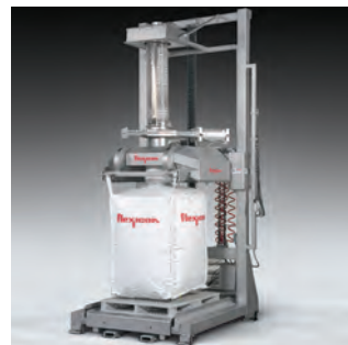
Sanitary SWING-DOWN® Bulk Bag Fillers offer stainless construction with continuous ground and polished welds, and a fill head that pivots away from its support structure, providing unrestricted access for high productivity and thorough wash down.
