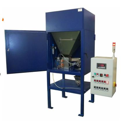
The BAYKON Gravimetric Color Feeder System is designed to weigh and feed granular materials at predetermined weights and time intervals. The system uses a electromagnetic vibro feeder to feed material into a weigh hopper mounted on a load cell, and than at a set time, disharge the product onto a second vibro feeder. By setting both target weighments and the disharge interval, accurate product feed rates can be achieved. The system consists of two unit. These feed cabinet and control panel.
