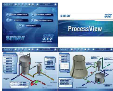
ProcessView Supervision / Operation System
