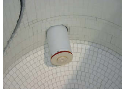
Grinding chamber with ceramic lining
