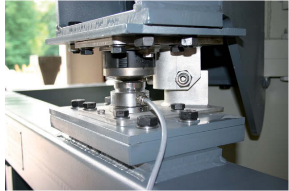
Load cell, mounted on CGS
