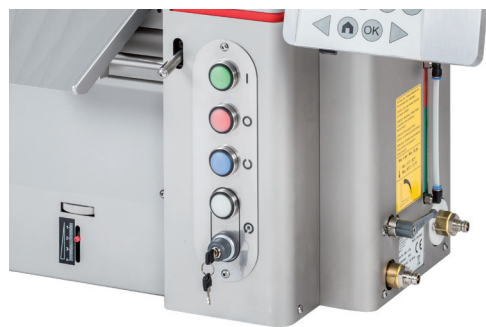
Control – Machine operation, scraper tension setting and connectors for temperature control
