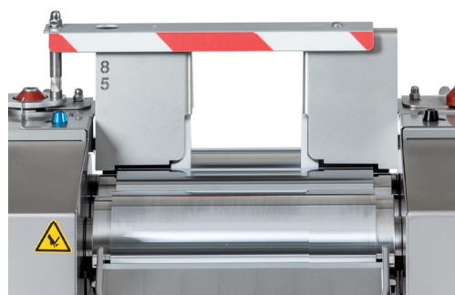
Safe and Operator friendly – Safety Bridge for 85, 170 and 200 mm working width
