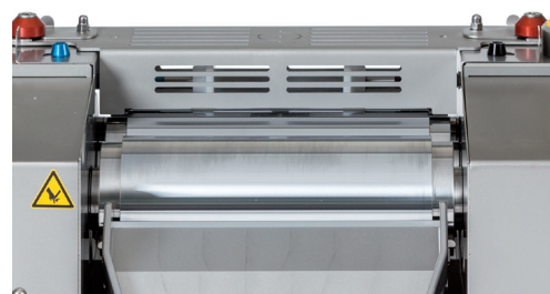
Nip-Cover – For press-out devices or small quantity batch processing
