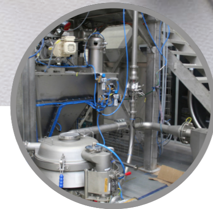
Inline Vibrating Sifter for pneumatic conveying
