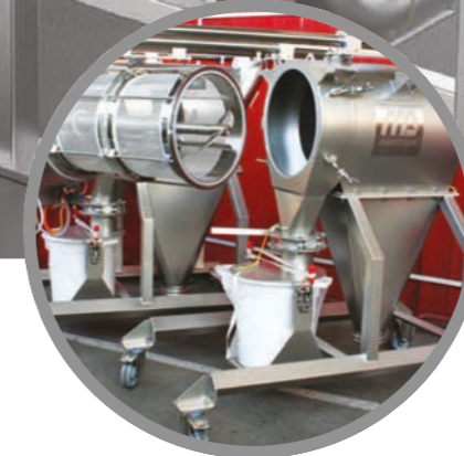
Centrifugal Sifter with Screen Inspection System
