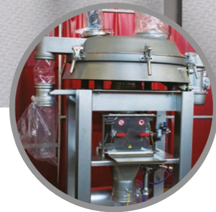
Vibrating Sifter with integrated magnet and sampling system
