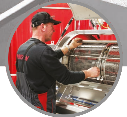
Centrifugal Sifter with Easy Access Wingdoors
