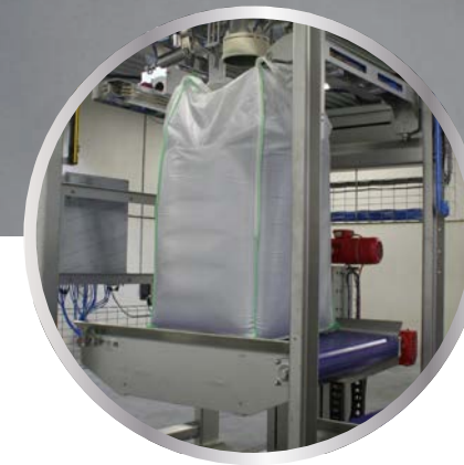
Electrically operated mechanical lifting table, no hydraulics are used.
