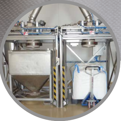
Filling system designed for multiple different types of container
