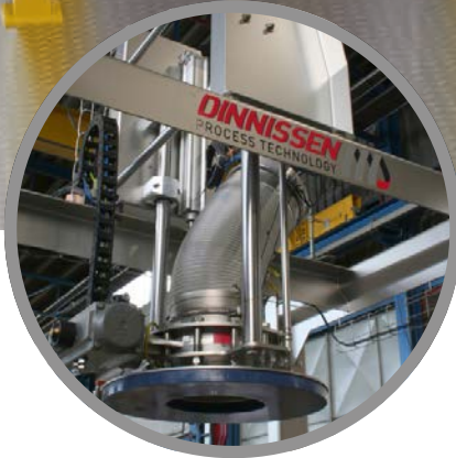
This flexible filling system connects to drums fully automatically
