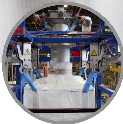
The Grab and Release System ensures that Big Bags are mounted safely and efficiently.
