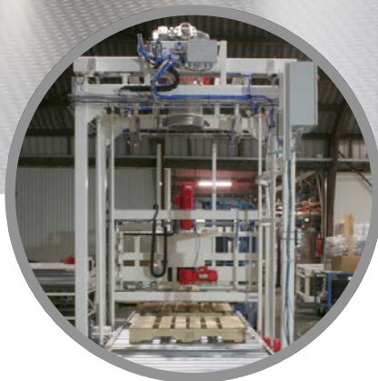
Big Bag Filling System with automated pallet supply and Big Bag Conveying.
