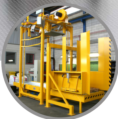
Big Bag Filling System with integrated pallet dispenser and palletizing system.
