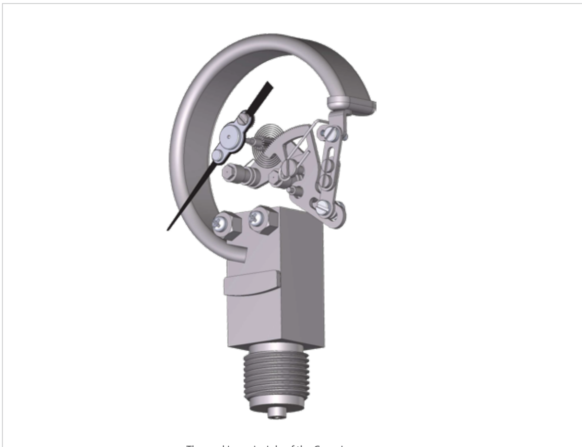
The working principle of the GeorGIN pressure gauge
