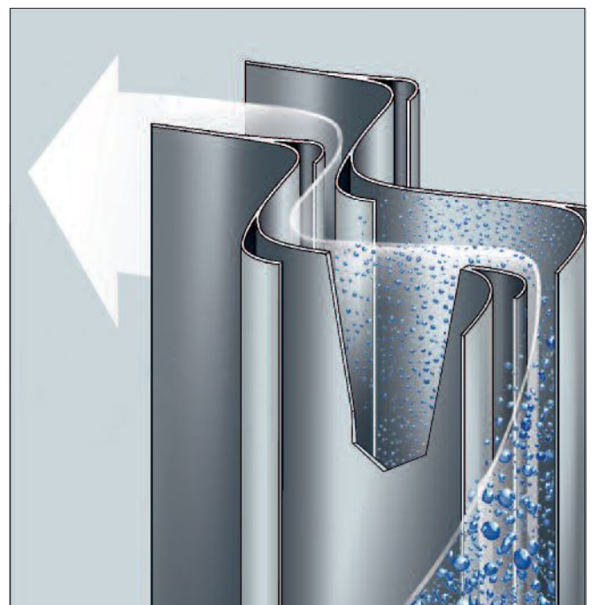
Functional principle of a horizontal separator
