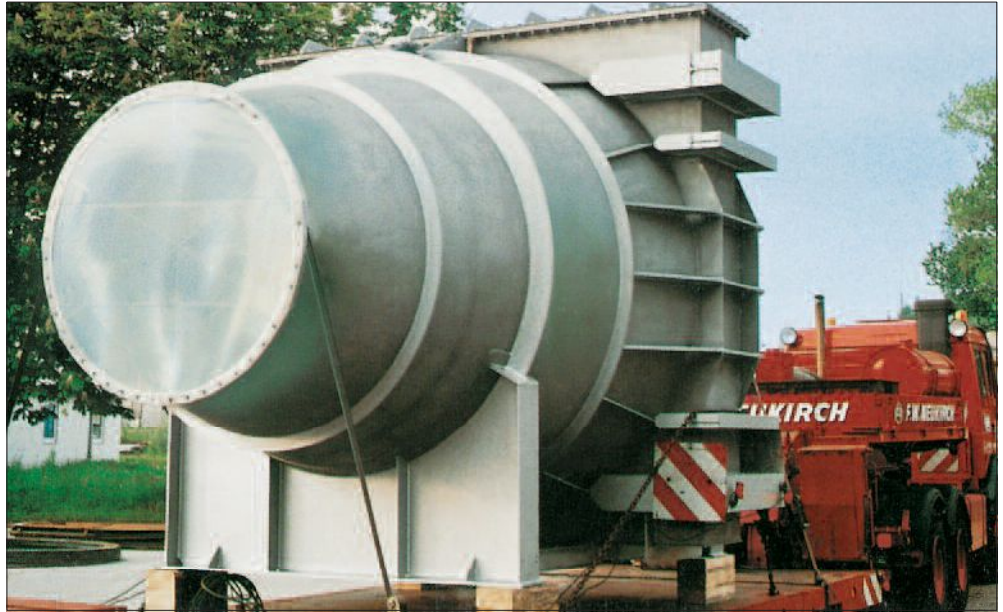
Droplet separator in a stainless steel housing
