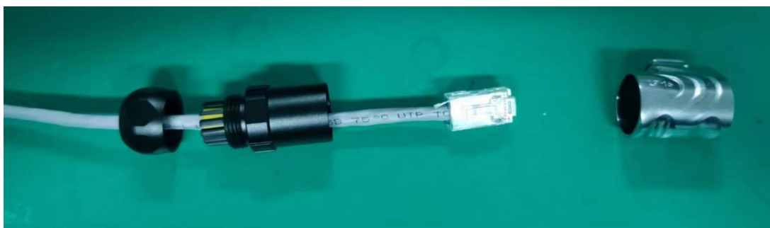
Chart 4-18 Waterproof quick-connect RJ45 data cable preparation
