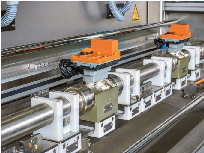
Multipoint wet calibration of the sensor modules
