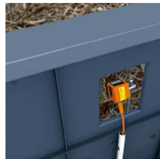
Level detection measurement in sugar cane delivery.
