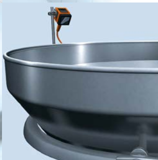
Level detection on a hopper.
