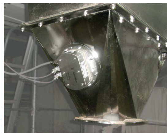
Sensor inside the wall of a buffer silo or a drop shaft
