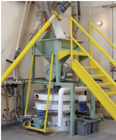
A 48 in. (122 cm) circular vibratory screener sifts up to 2,000lb/hr (907kg/hr) of durum granular flour. Auger conveyor transports a small amount of recycled, ground pasta to the feed hopper.
