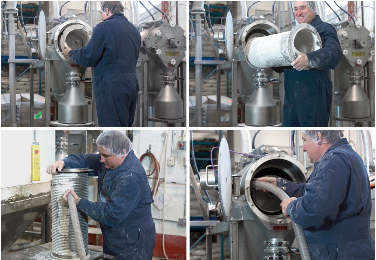
Quick cleaning: Operator opens end plate, removes basket, and cleans basket and sifter interior in 10 minutes.
