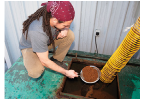
Dewatered grain (stillage) having approximately 80% moisture content is utilized for animal feed.
