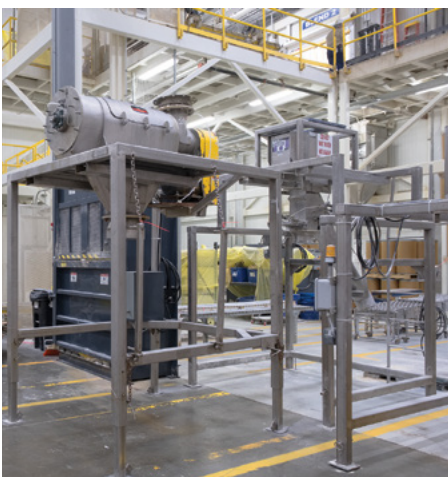
CENTRI-SIFTER centrifugal sifters screen ingredients to meet particle size requirements and maintain product quality. At right, 50 lb (23 kg) bags of ingredients await sifting.
