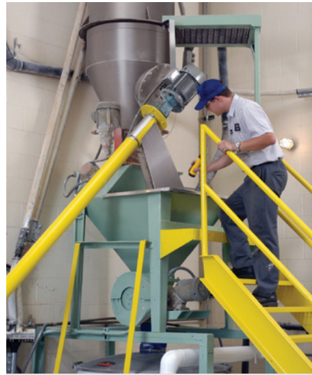
Operator checks flow of durum granular flour and recycled ground pasta into feed hopper, rotary airlock and 48 in. (122 cm) screener below.
