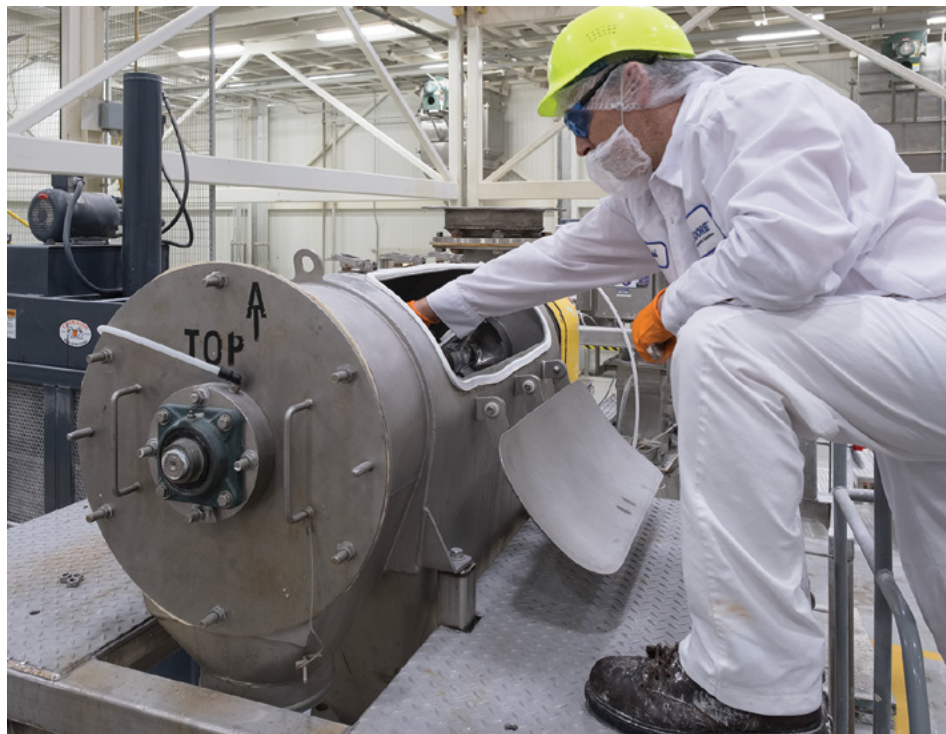
A hinged door with safety interlock provides interior access for cleaning, inspection and screen changes.
