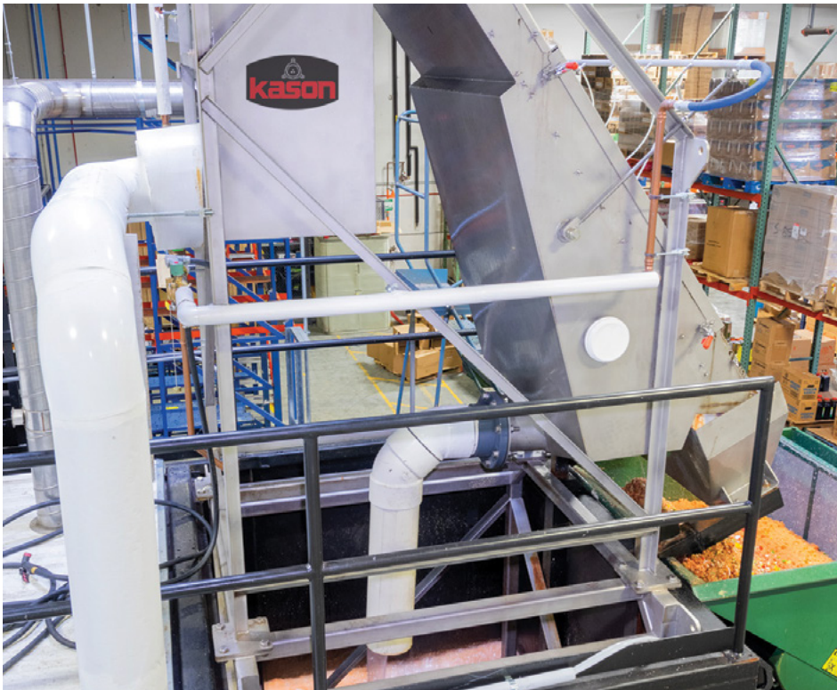
Wastewater is pumped onto the dewatering sieve which separates solids at high rates without the use of power.
