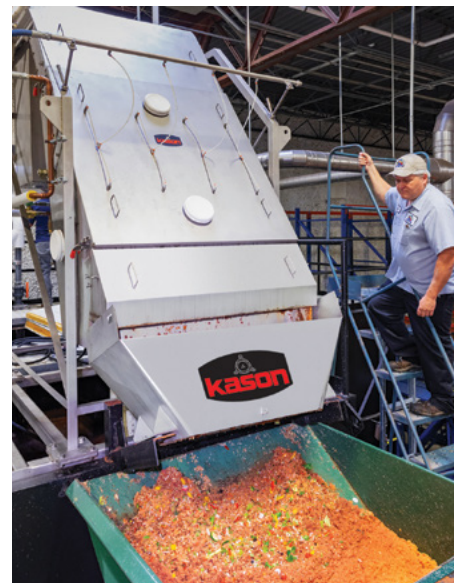
Wastewater flows over an inclined screening deck that captures peelings, stems, foreign objects and debris as small as seeds.
