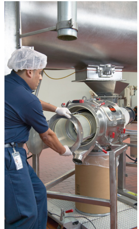
The three-bearing cantilevered shaft of the Quick Clean CENTRI-SIFTER screener enables the operator to open a hinged end cover and remove the screen cylinder and paddle assembly for rapid screen changes and cleaning during frequent product changeovers.
