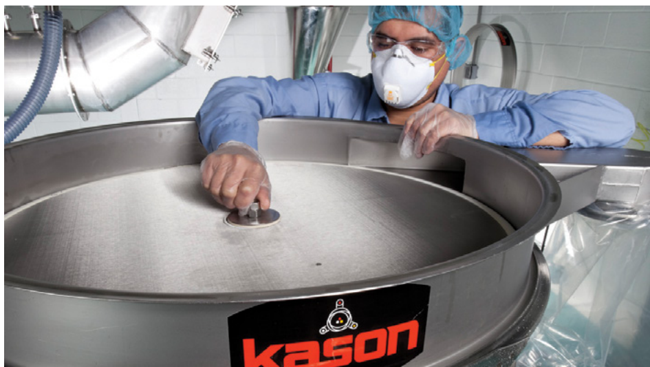
A Kason vibratory screener with circular 80 mesh (178 µm, 0.0070 in.) screen is inspected between production batches of fragrance powders.
