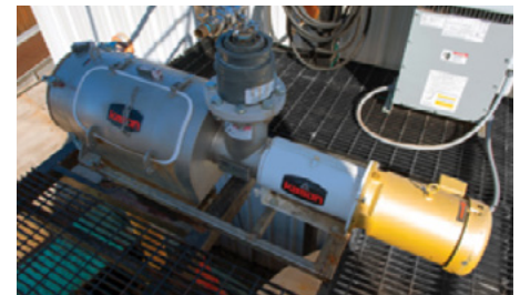
The CENTRI-SIFTER centrifugal sifter at the distillery runs at a higher voltage than normal in order to screen heavy, sludgy stillage.
