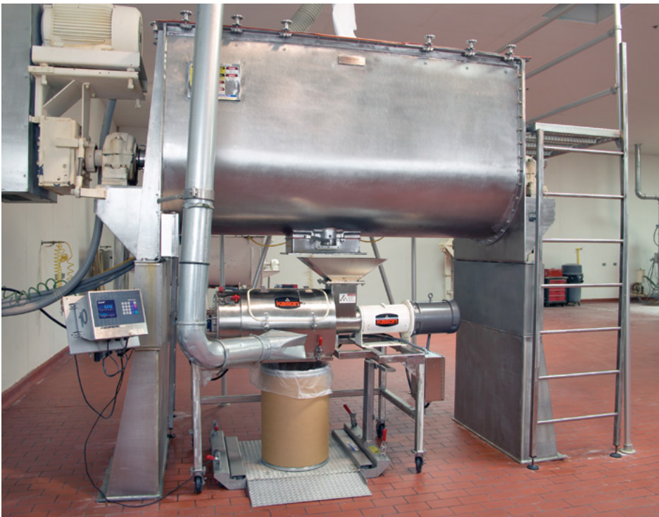
A Quick-Clean CENTRI-SIFTER centrifugal screener fits the restricted space below an 80 cu-ft (2.2 cu-m) capacity blender, sifting flavor powders at high rates.
