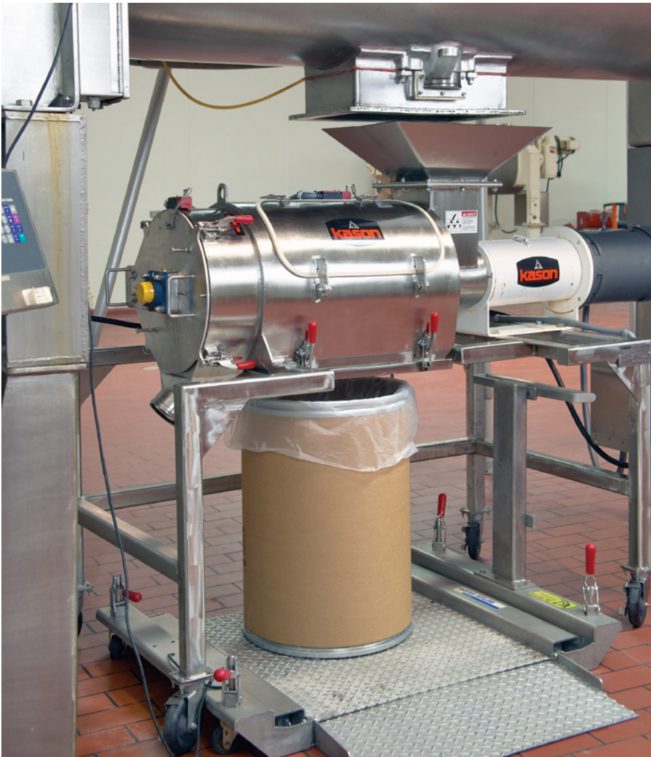
The Quick-Clean CENTRI-SIFTER screener gravity-discharges into 100-lb (45-kg) capacity fiber drums, and can be rolled to a cleaning station and other blenders.
