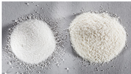
Material before (left) and after being moisturized, agglomerated and dried in the circular fluid bed processor.
