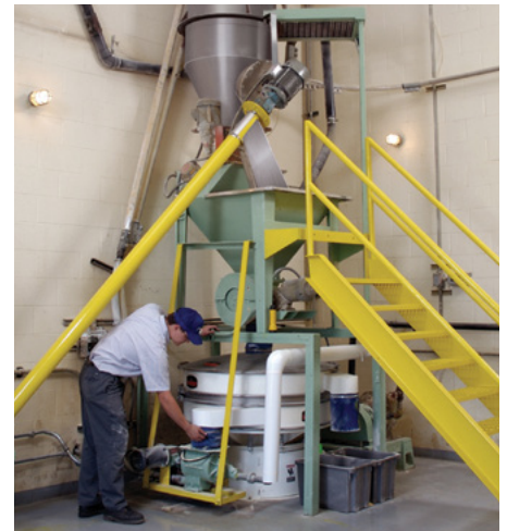
A 48 in. (122 cm) circular vibratory screener replaced a vintage gyratory sifter, decreasing waste and saving time and labor in re-screening rejected material.
