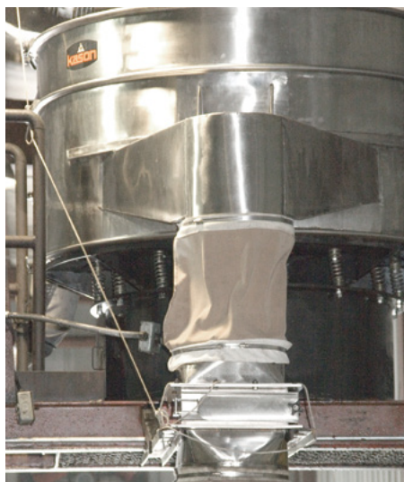
Rotation of the screener's motor produces both vertical and horizontal vibration of the screening deck. Vertical vibration causes sugar particles to pass through apertures in the screen at high rates. These particles exit the screener through a discharge spout. Horizontal vibration moves oversize particles to the periphery of the screener, where they exit the device through a chute.
