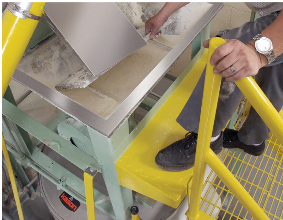
Operator checks flow of durum granular flour and recycled ground pasta into feed hopper, rotary airlock and 48 in. (122 cm) screener below.
