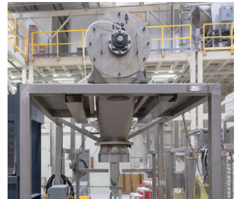
Centrifugal sifting maintains high throughput and product integrity at PacMoore's Mooresville, IN plant. Screened product gravity-discharges through a central chute.
