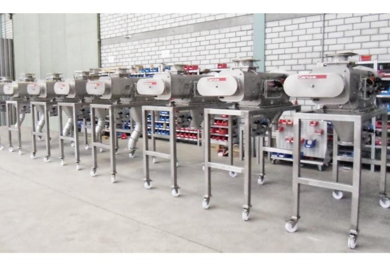
Gericke sifters have been designed and developed for the .optimisation of these sifting applications. The basic principles of centrifugal sifting provides high level performance and optimum separation with a minimal footprint.
