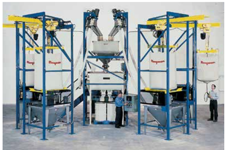
This turnkey, Gain-in-Weight Batching System conveys material from four Flexicon bulk bag dischargers to a weigh hopper which discharges into a blender. During the blending operation, a subsequent batch is being weighed by the hopper, thereby reducing cycle times. In this case, blended batches are discharged directly into shipping containers.
