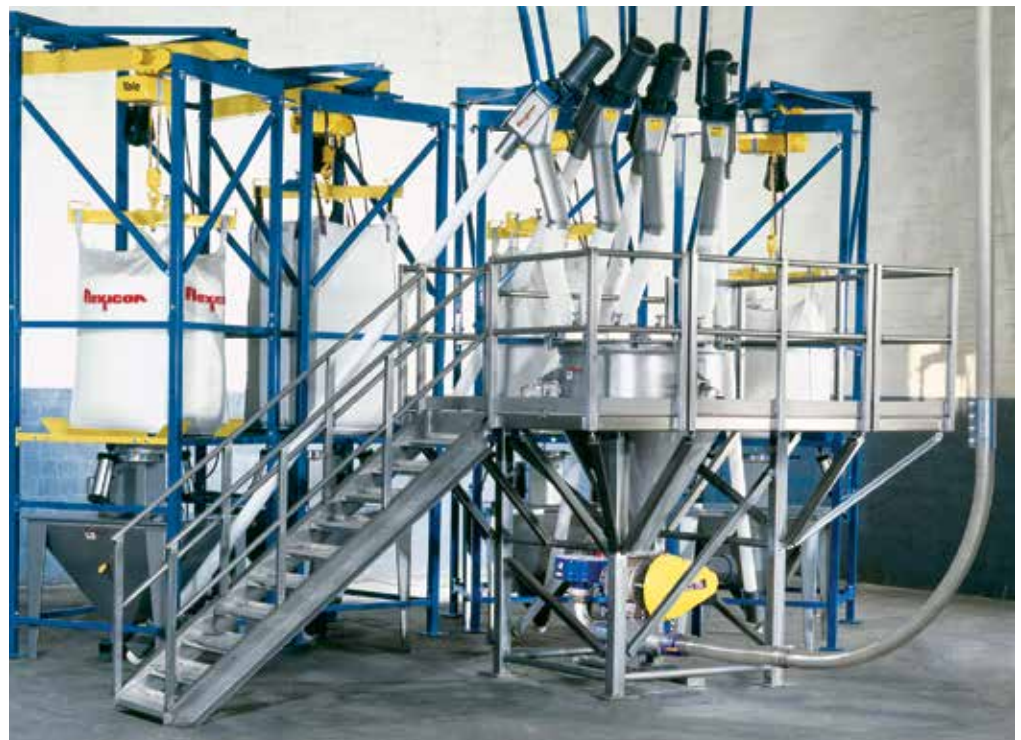
This Automated Weigh Batching System conveys material from Flexicon bulk bag dischargers via Flexicon flexible screw conveyors to a weigh hopper mounted on load cells at mezzanine level. Weighed batches are automatically discharged through a rotary airlock valve into a Flexicon Pneumatic Conveying System, transporting the pre-weighed batch to a blender.
