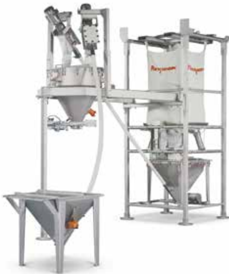
This Gain-in-Weight Batching System allows automated weighing of a major ingredient supplied in bulk bags, and a minor ingredient dumped manually. The central weigh hopper's load cells transmit weight gain information to a controller that starts and stops the conveyors to weigh each material in sequence, and actuates a slide gate valve to discharge the weighed batch.
