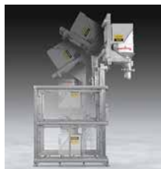
Sanitary TIP-TITE® Drum Tippers allow loading, sealing, tipping and discharging of drums with no dusting by forming a dust-tight seal between a drum discharge cone and a gasketed receiving ring fitted to existing process equipment or the lid of a hopper.
