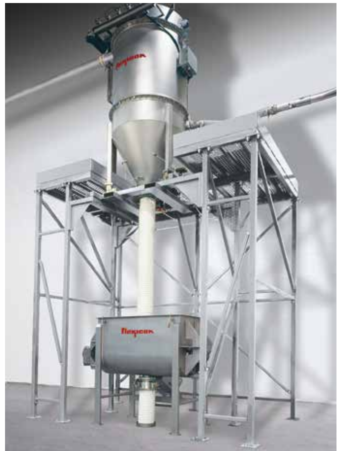
This modular vacuum receiver features a rugged clamp-together design that facilitates rapid disassembly for filter maintenance and cleaning. Whereas conventional filter receivers employ multiple smaller elements, this design employs a single, large diameter filter cartridge, and offers an ideal solution for low-throughput-rate, short-distance pneumatic conveying applications.
