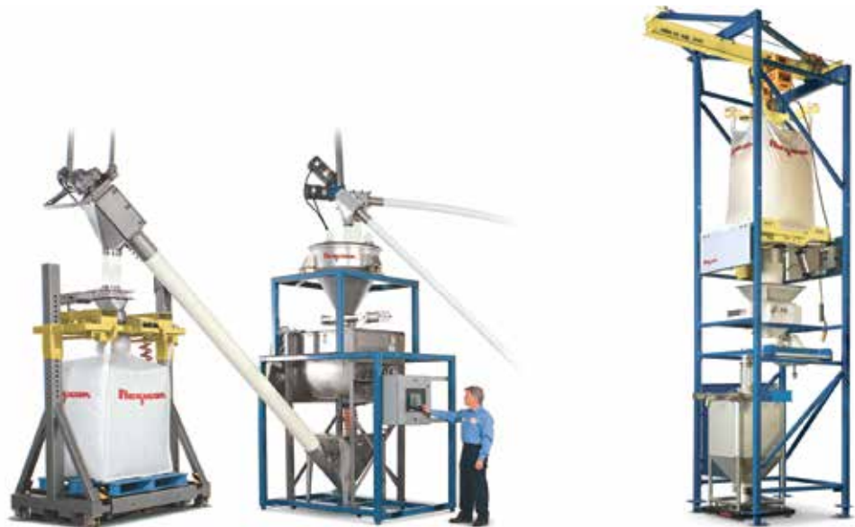
Flexicon's Self-Contained, Gain-in-Weight Batching and Blending System conveys bulk ingredients from multiple upstream sources, weigh-batches, blends and discharges the material into a surge hopper, and transports it to a TWIN-CENTREPOST™ Bulk Bag Filler. The system is offered with Flexicon Flexible Screw Conveyors (shown) or PNEUMATI-CON® Pneumatic Conveying Systems.
