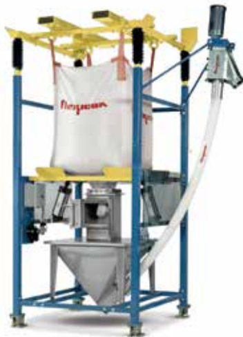
Loss-of-Weight Batching Systems discharge one or more bulk bags while weighing the material and conveying the batch directly to a common hopper, blender, conveyor, shipping container, or any process vessel—automatically and accurately. Load cells transmit the amount of weight lost to a controller, which stops the conveyor once the target batch weight has been reached.
