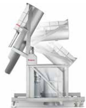
Open Chute Drum Tipper offers a low cost method of discharging free- and non-free-flowing bulk solids when dust generation is not a concern. Discharges directly into process equipment or optional hoppers equipped conveyor adapters or universal flanges.
