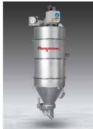
This modular vacuum receiver features a rugged clamp-together design that facilitates rapid disassembly for filter maintenance and cleaning. Whereas conventional filter receivers employ multiple smaller elements, this design employs a single, large diameter filter cartridge, and offers an ideal solution for low-throughput-rate, short-distance pneumatic conveying applications.
