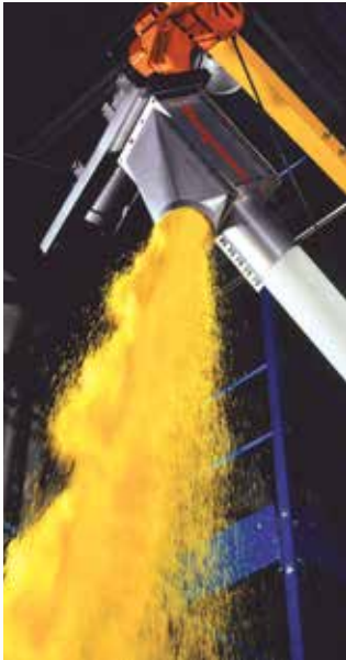
High capacity flexible screw conveyor with downspout removed to demonstrate flow of material.
