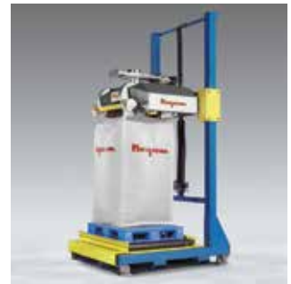
The bag connection frame has pivoted to horizontal position, the fill head is raised to "bag fill" position, and the bag has inflated to remove creases.
