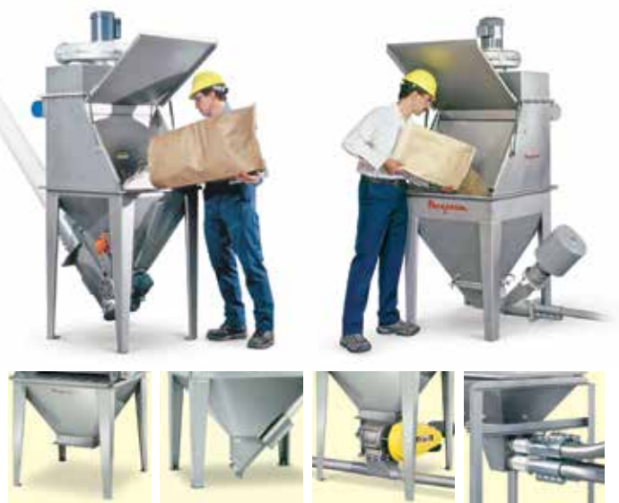
The hoppers of Flexicon Bag Dumping Stations are offered with outlets configured for: (left to right) direct connection to process equipment, flexible screw conveyor charging adapters, rotary airlock valves with flow-through adapters, and non-flow-through pick-up adapters for multiple conveying lines.
