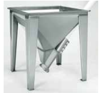
Divergent angles of Flexicon's patented high flow hopper design reduce the ability of non-free-flowing materials to establish a bridge between the hopper sidewalls, instead causing material to topple and flow toward and down the steep backwall, increasing the flow of bulk materials while decreasing residual material in the hopper.
