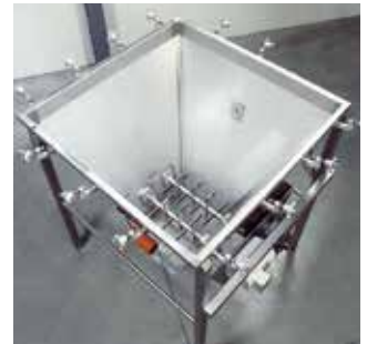
Flexicon offers a multitude of mechanical and pneumatic hopper accessories to promote the flow of poor-flowing or non-free-flowing materials. This hopper features dual agitators with interlocking paddles that de-agglomerate bulk material, promoting void-free charging of mechanical conveyor intake adapters.
