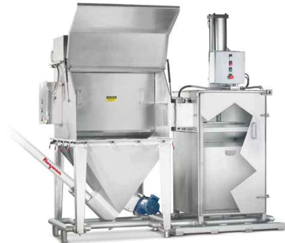
Self-contained Bag Dump System integrates a dust collector, flexible screw conveyor and bag compactor on a skid, streamlining installation and allowing easy relocation. The entire airtight system is under negative pressure, containing dust when bags are dumped, as well as when empty bags are pushed through the chute and compacted.
