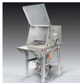
Sanitary Bag Dump Stations with optional dust hoods on rocker arms raise the hood for easy separation and wash down of the gasketed seam—and for removal and wash down of the interchangeable dump screens. Dust collection prevents contamination of personnel and plant environment.
