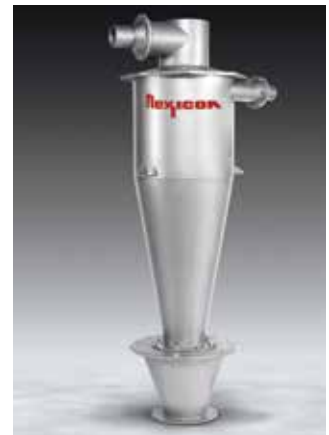
Unlike filter receivers, cyclone separators require no filters to separate solid particles from the gas stream, instead relying on cyclonic action alone. An air stream containing material enters the separator at a tangential angle and is spun rapidly, creating a circular flow that imparts centrifugal force to the particles which strike the wall of the cyclone and fall through a bottom outlet, into a process vessel.
