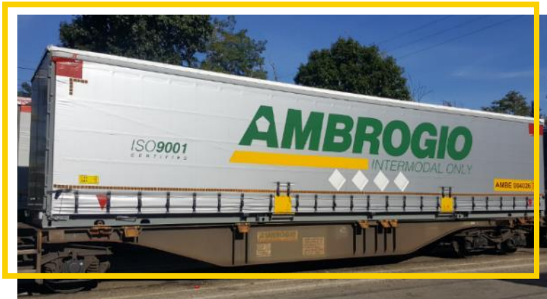
13,60m swap bodies, tautliner with sliding roof, with or without side drops
