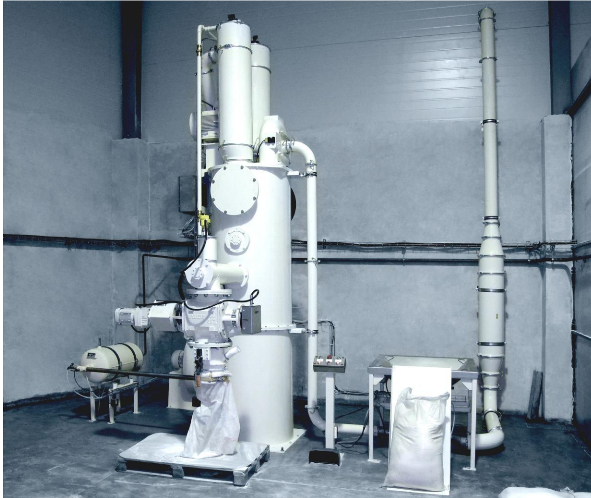
REKORD BT-ex Sugar Grinding Plant for 1200 kg/h of finest powder sugar
