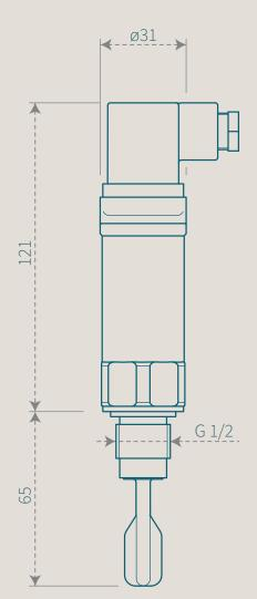
Suitable for high temperature liquids **up to 150°C**.
