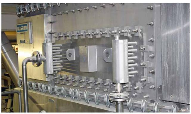
Tubular heat exchanger installed in fluidized bed dryer
