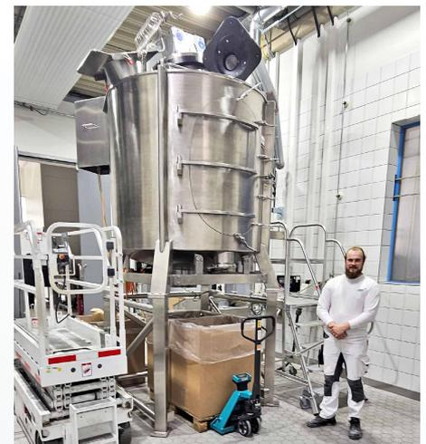
The Gyraton® test mixer is suitable for batches of up to 3 m³. Gas-tight, hygienic, universally applicable.
