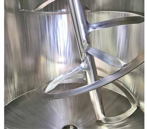
The base has the shape of a dome segment. The mixing goods are mixed without dead space. If desired, they can even be completely discharged using ComDisc®.
