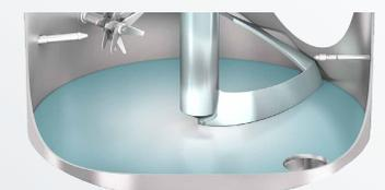
Mixing unit rigidly mounted: The center receives less flow. Therefore, the rotation frequency should be more than 4 to 7 rpm.
