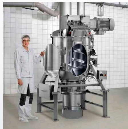
Type KS 400 with 2 Clever-Cut® designed inspection doors
