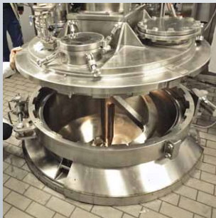
Headplate lifts automatically
