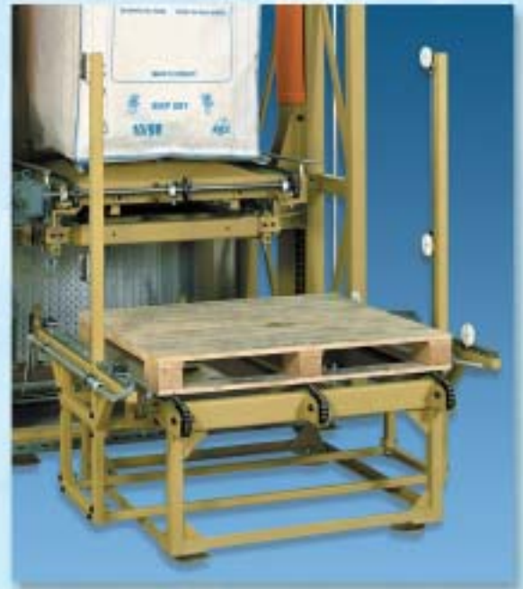
Automated pallet drive-in and bag drive-out system
