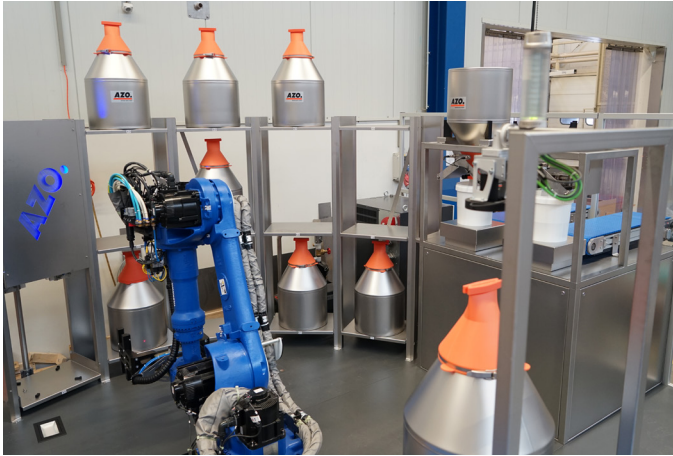
The robot removes the dispensing and storage units with the component specified in the formulation from the storage module for raw materials.
