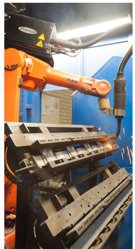
Above: Rewag factory of AVK Nederland BV where REPICO® is produced Right: Robotic welding in the Rewag factory
