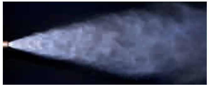
Spray pattern of the MasterNOx® nozzle 30°
