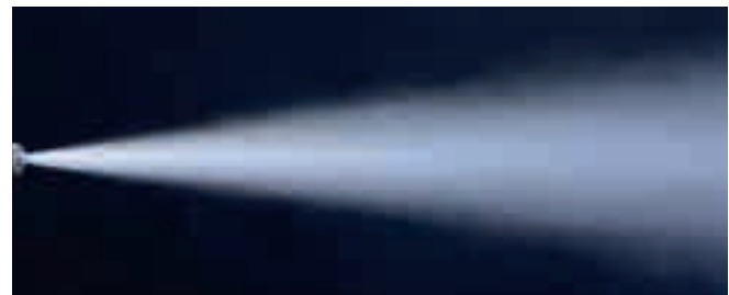
Spray pattern of a Laval nozzle
