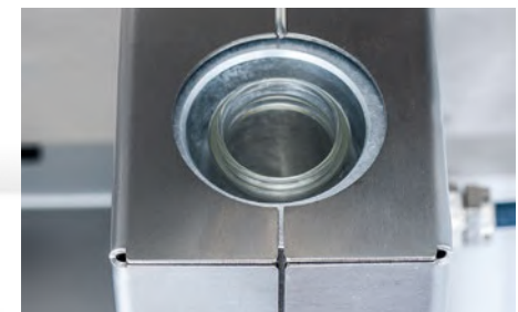
Heating from sample vial via the sample loop and tubing to the first column.
