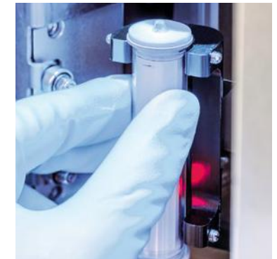
Insertion of columns - sensors check, if columns match with method input
