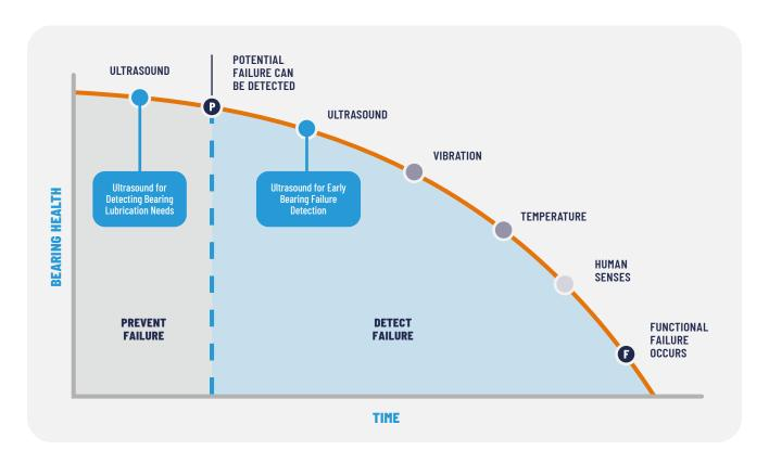
While most technologies identify faults and cracks only after they've progressed, ultrasound excels by spotting these issues in their earliest phases, including crucial lubrication needs.
