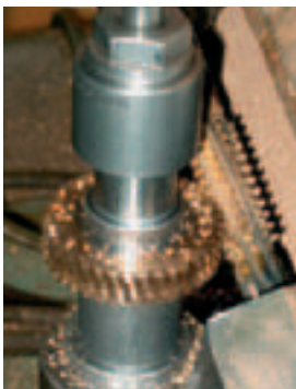
Machining of worm wheel gearing with OFA 16 NC hobbing cutter.
