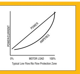
At low loads, motor amperes do not change much with small changes in loads. Small signal changes can cause false trips or allow equipment to operate below the desired minimum operating point.
