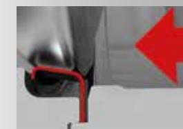
Bi-directional tightness The medium-pressure supports the flexible metal sealing-ring to follow the disc during the transition to be compressed in a way that it is almost equal to both flow directions.
