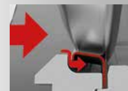
Bi-directional tightness The medium-pressure supports the flexible metal sealing-ring to follow the disc during the transition to be compressed in a way that it is almost equal to both flow directions.
