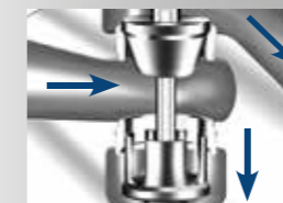
Variable: diverting plug.
