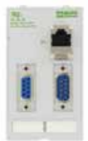
RJ45; SUB-D9; SUB-D9 1 × RJ45, 8-pole. metal, CAT5e (socket/socket) 1 × SUB-D9 (socket/socket) 1 × SUB-D9 (pin/pin) Order No. 20.90 10 62
