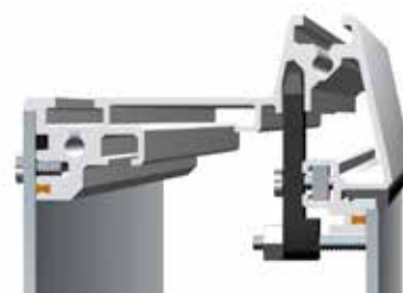
Front panel installation with stud bolts
