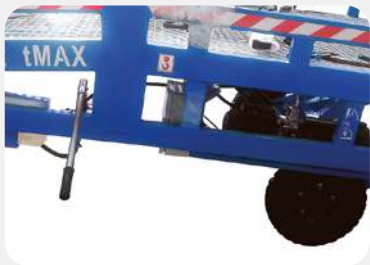
ELECTRIC HYDRAULIC STATION AND MANUAL PUMP
