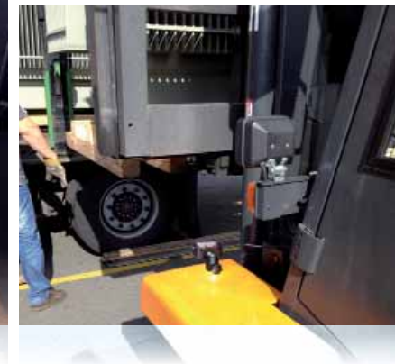
Camera-assisted truck loading.
