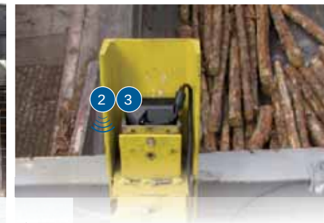
MC3000B for monitoring the filling level of a wood container.
