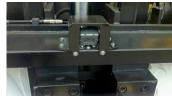
A carriage mounted camera is lifted simultaneously with the load.
