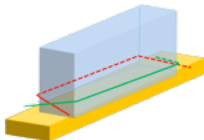
horizontal half-loop lashing at not ow case
