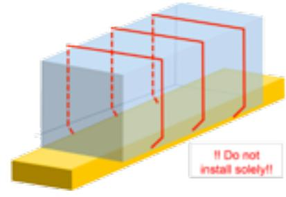
top-over lashing, friction lashing
