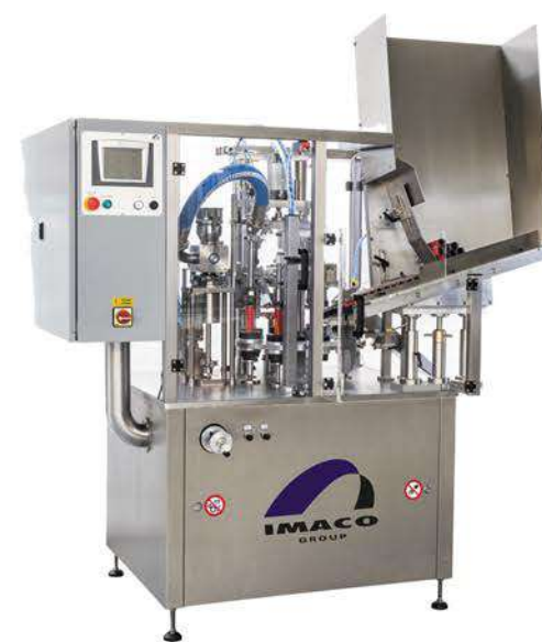
Tube filling system
