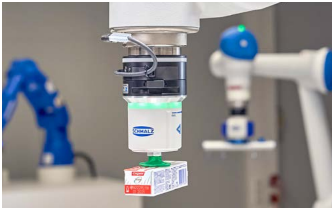
Handling Set ECBPMi MATCH for automated small parts handling
